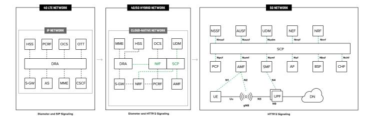
**Figure 3:** Mobile core signaling evolution
