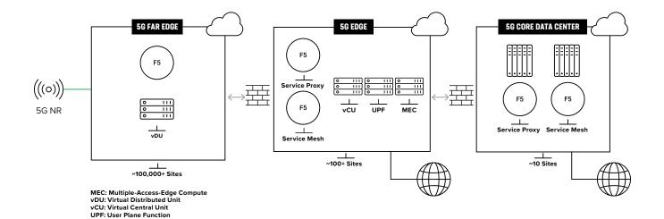
**Figure 12:** F5 infrastructure solution scaling capability
