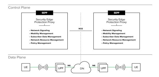
**Figure 7:** Security Edge Protection Proxy (SEPP)
