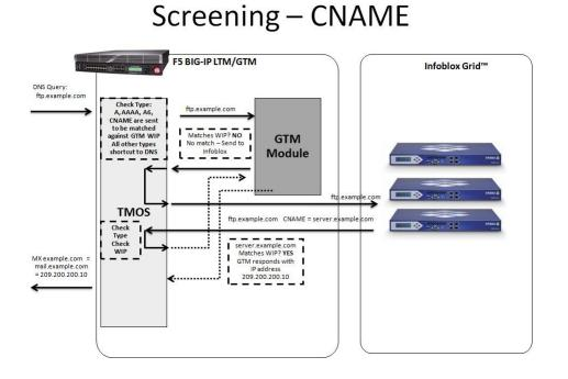
An illustration of the request flow when the initial record type is an A-record.
