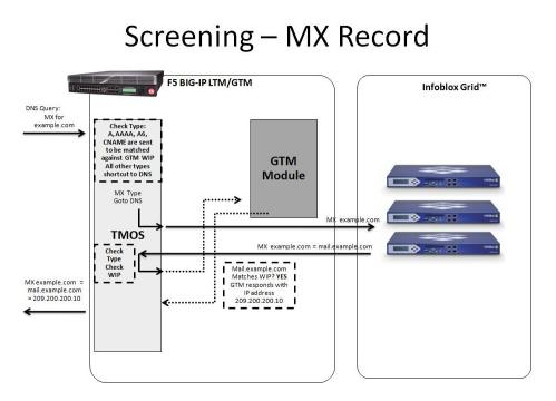
A good illustration of the integrated capability of a BIG-IP GTM screening architectures is when an MX record is requested. BIG-IP GTM only has the WIP list and configuration for processing the WIP queries. All zone records are maintained on the Infoblox appliances. The requests flow through the system in the following steps:
