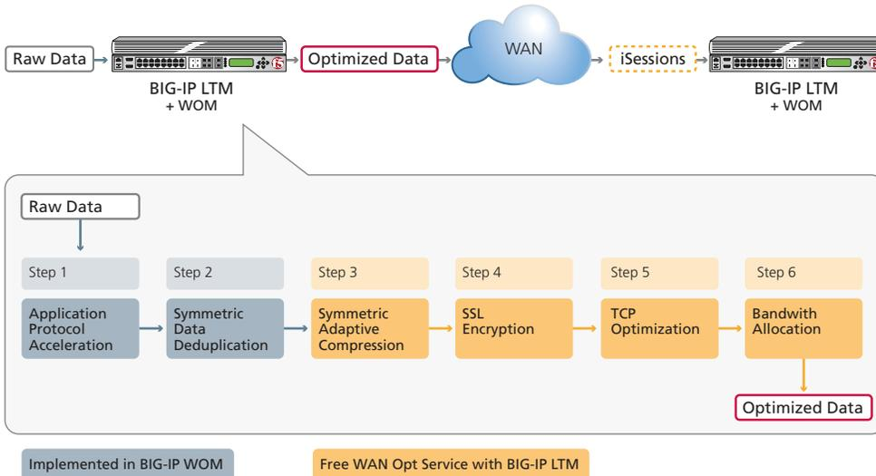
BIG-IP WOM on either end of your connection increases bandwidth utilization, encrypts the data being transferred, and speeds your remote disk-to-disk backup timeframes.
